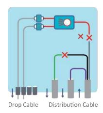
For card type splitter type box, the distribution cable is spliced to the input pigtail of the splitter and connect with preconnected drop cable (or terminated with field assembly connector)
